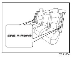
The rear side air bags are stowed in the covers at both door-side ends of the rear seatback. The words "SRS AIRBAG" are molded into each of the seatback ends.
